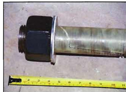
Figure 4: Bolt sleeve failure due to shear stresses.
